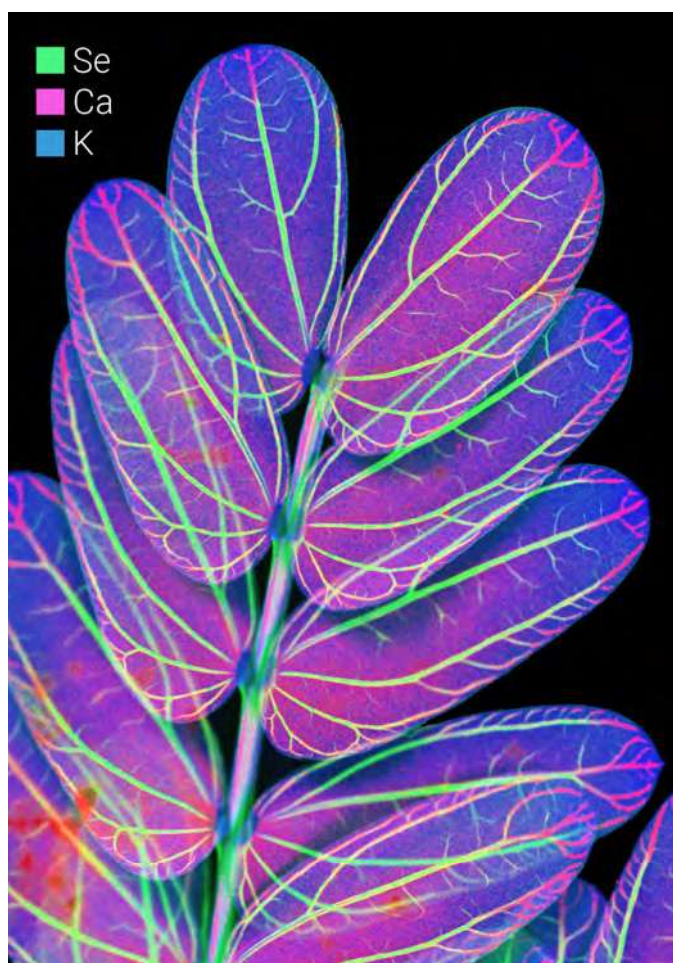
MicroXRF elemental map of K, Ca and Se in a hydrated fully opened leaflet of Neptunia amplexicaulis (image courtesy of University of Queensland).
