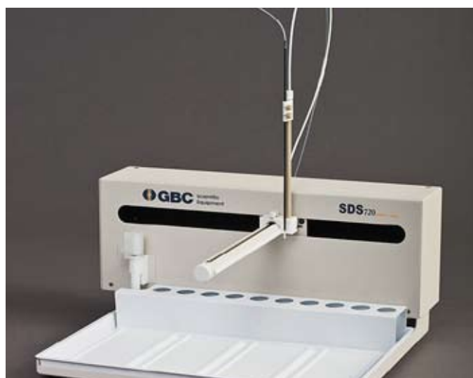
SDS720 allows 10 standards and 360 samples to be analysed.
