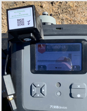
MX908 outfitted with an Aero and co-located with a particle counter to provide ground truth measurements of the aerosol plume.
