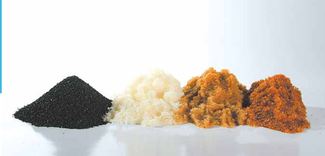
ACTIVATED CARBON, ANION, MIXED BED AND CATION EXCHANGE RESINS (FROM LEFT TO RIGHT)
