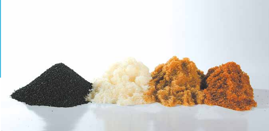
ACTIVATED CARBON, ANIONS, MIXED BED AND CATION EXCHANGE RESINS (FROM LEFT TO RIGHT)
