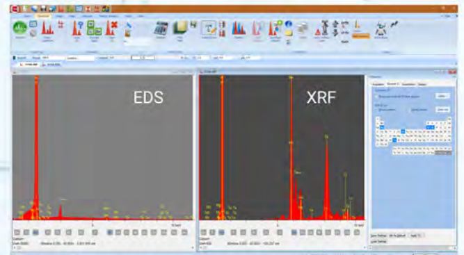
Comparison of SEM/EDS and SEM-XRF for a Al-Ta-Mn alloy specimen showing that X-ray excitation fully resolves all elements, allowing accurate quantification by standardless FP.
