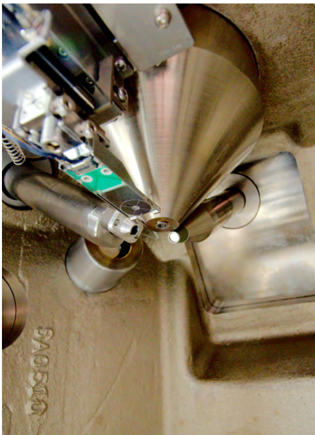
Interior of SEM showing (from left to right) the EDS detector nose, the SEM pole piece and IXRF's fX SEM small spot X-ray source.
