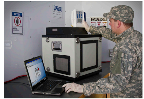
Figure 6. Griffin X-Sorber docked with Griffin G460 GC/MS for rapid sample identification
