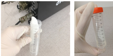
Figure 3. Particle Extraction from DFU into Liquid
