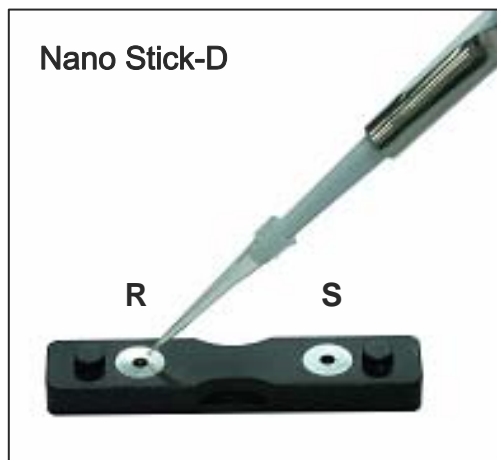
Pipette the blank and the sample in their respective port
