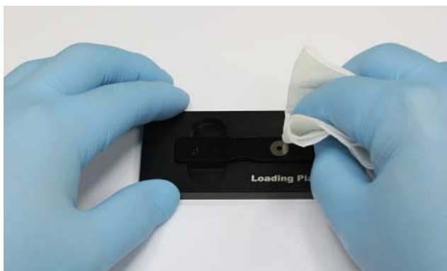
5. Clean the sampling area for next sampling
