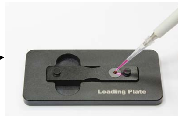
6. Pipette the Sample
