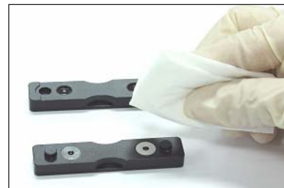
Clean both ports for next sampling
