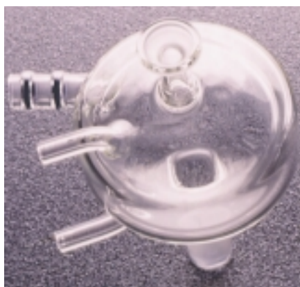
Jacketed spraychamber for below-ambient temperature aspiration of volatile organic matrices
