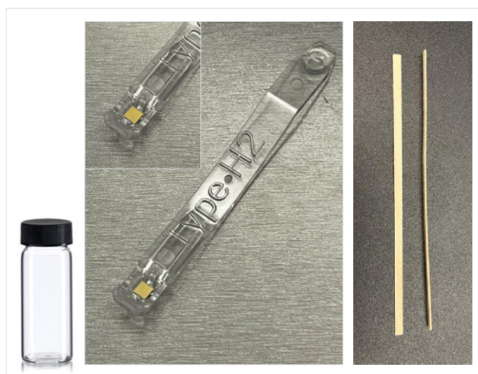
Figure 1. Items that come with the Type H2 Kit: a small vial for methanol, the Type H2 stick with the metal substrate, and wooden spatulas for sampling.
